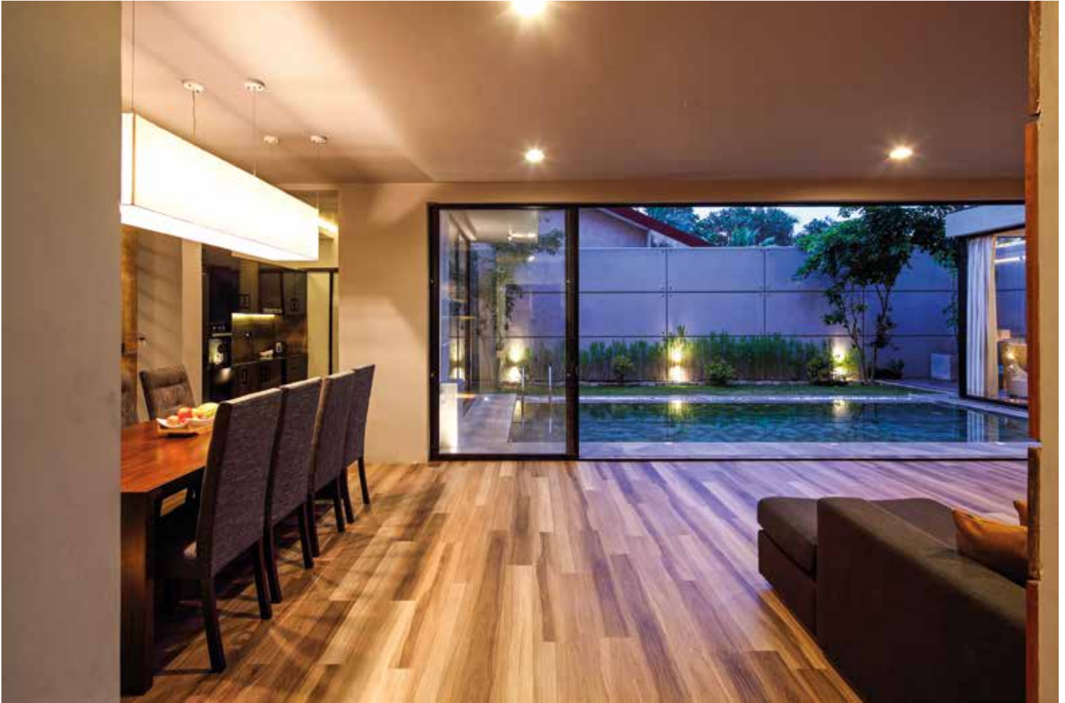
The space allocation has ensured the internal thermal comfort levels are maintained as the swimming pool will facilitate evaporative cooling to the inside spaces.
